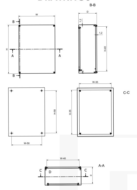
Drawings above refer to Control Station with bolted cover. For the drawings of hinges of Control Stations ask to info@ce2k.com.
